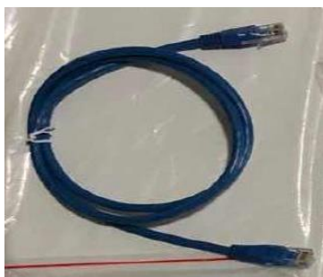
Figure 51 – Câble de communication entre batteries AZZURRO 5000
